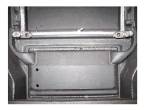
6. Place the new bypass cover into position. Apply anti seize compound to the bolt threads. Swivel the retainers back into position, and secure them with the bolts provided.
