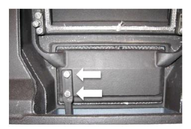
5. Completely remove the front bolt from each of the bypass retainers, and loosen the rear bolt using a ½" wrench. It may be necessary to remove the center ½"-20 x 1" bolts, (loosen lock nuts first) using 7/16" wrench. Twist the retainers out of the way and remove the bypass cover.
